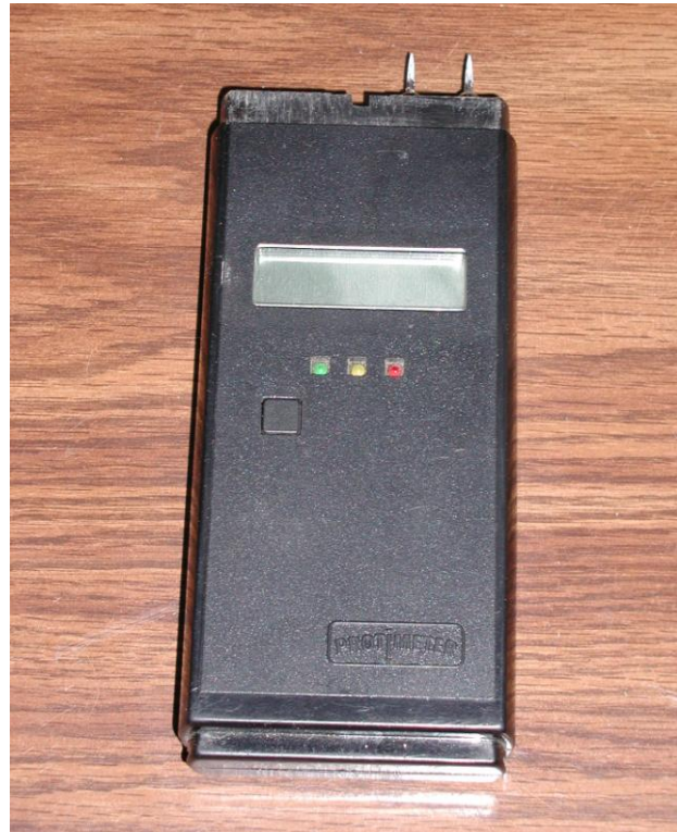
One type of Wood Moisture Meter. The probes at the top of the picture are pushed into the wood.
